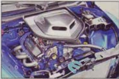
408 stroker was built by Southeast Performance in Tampa, FL. The 10-1 motor puts out a dyno'd 415 HP to the wheels plus another 150 ponies from squeeze. Intake is a 4-8oz M-1 with SGM throttle body. Ignition is MSD 6AL Digital. Exhaust is GSM headers and Spintech mufflers with cats deleted.
